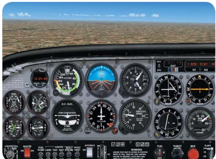
**GETTING READY TO TURN ONTO THE 053 RADIAL FOR THE BOILER VOR. NOTICE THE HEADING INDICATOR AND THE BEARING RING ON THE VOR 2 RECEIVER. AFTER THE TURN, THEY'LL BOTH READ THE SAME**
