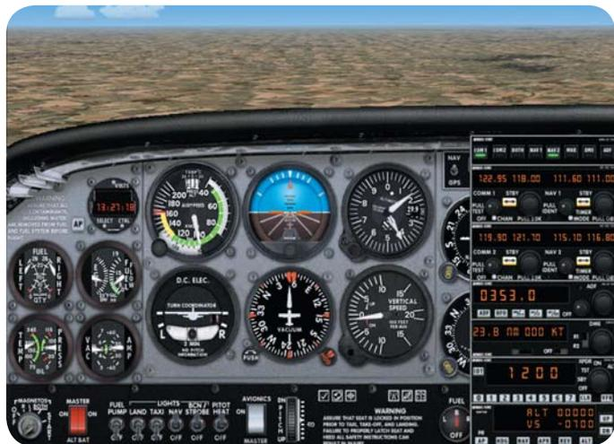
**RESETTING THE NAV 1 RADIO TO 111.60 AS WELL AS SETTING THE VOR 1 OBS SO IT WILL TRACK THE 311 RADIAL OUT OF KANKAKEE**
