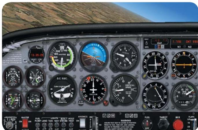
**ROLLING OUT ONTO THE 311 RADIAL. NOTICE THE DME IS STILL SET TO THE BOILER VOR. THE HEADING INDICATOR AND THE VOR 1 BEARING WILL READ THE SAME AT THE COMPLETION OF THE TURN.**
